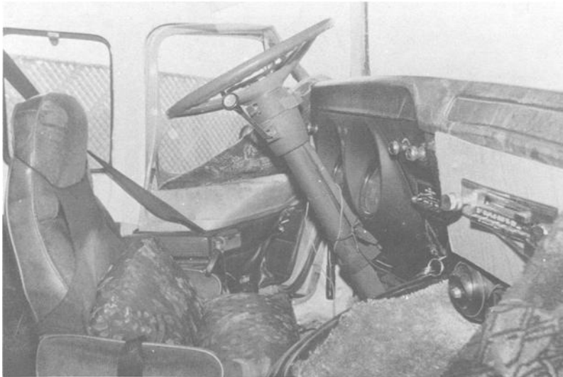
FIG. 4— Van's steering column and steering wheel rim were pushed upward and backward at impact. Note that steering wheel rim is near top of driver's seat and at level of driver's neck. (Wide angle lens: 28 mm).
