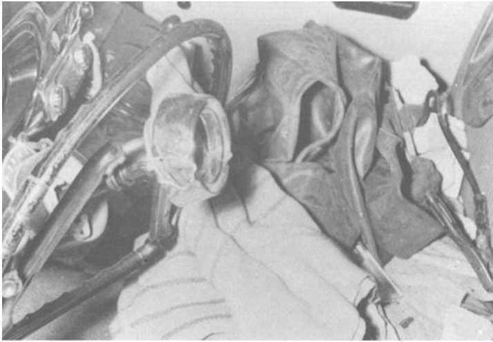
FIG. 9—Downward and backward displacement of steering rim after head-on collision. Compare steering column with chest imprint (Fig. 7) and location of rim with laryngeal injuries.
