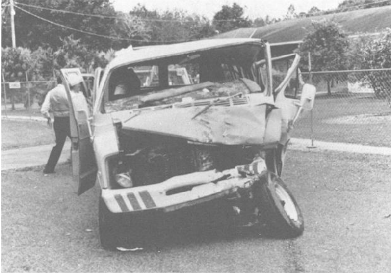
FIG. 3— Inward crush of van's left front after head-on collision.
