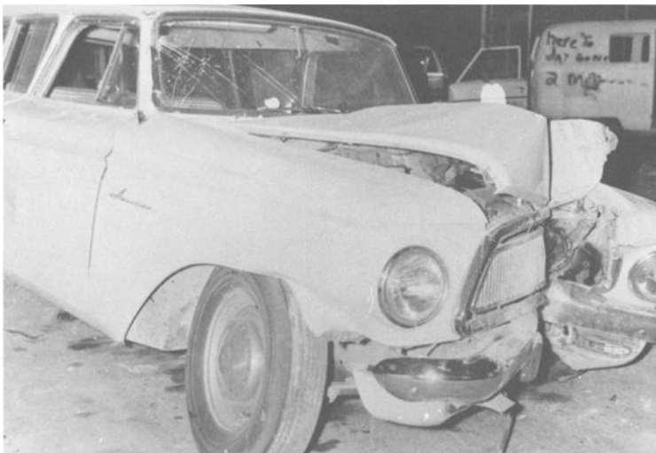
FIG. 8—Inward crush of front of vehicle after head-on collision with power pole.
